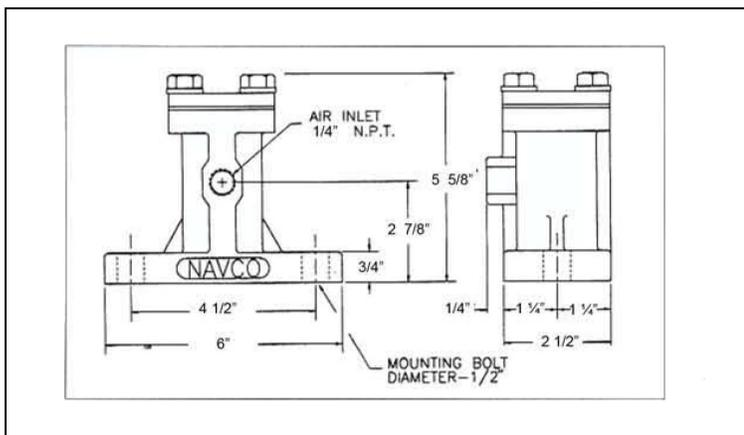
The Stainless Steel NAVCO BH 1<sup>1</sup>/<sub>4</sub> is a Pneumatic Piston Vibrator designed to provide reliable performance. Stainless Steel makes for easy cleanability which is important for food and pharmaceutical applications. This vibrator is ideal for ensuring consistent material flow of light duty bulk material in any environment.
