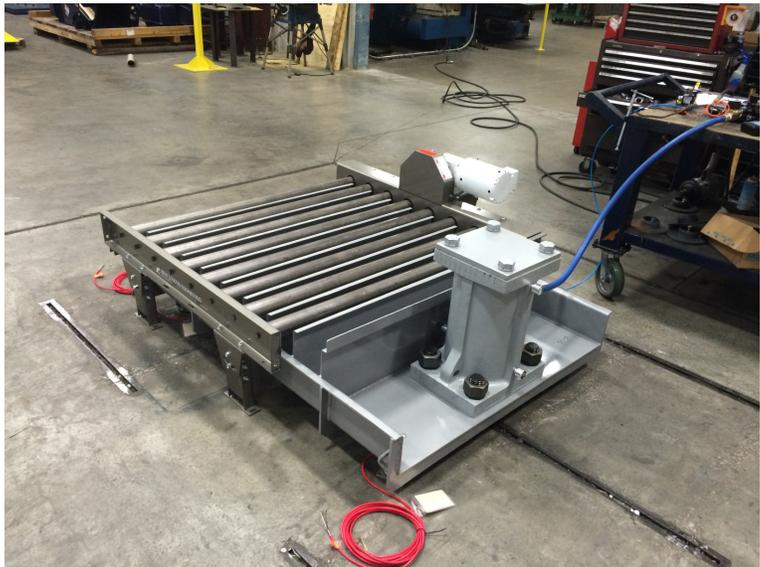
Based on in house materials test, a high stroke, low frequency vibration forcing function was decided upon to consolidate this difficult material.
