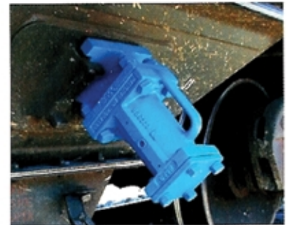
NAVCO HCP Vibrator ensures material flow from rail cars.
